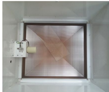
Step 2. Remove lamp and lamp holder.
